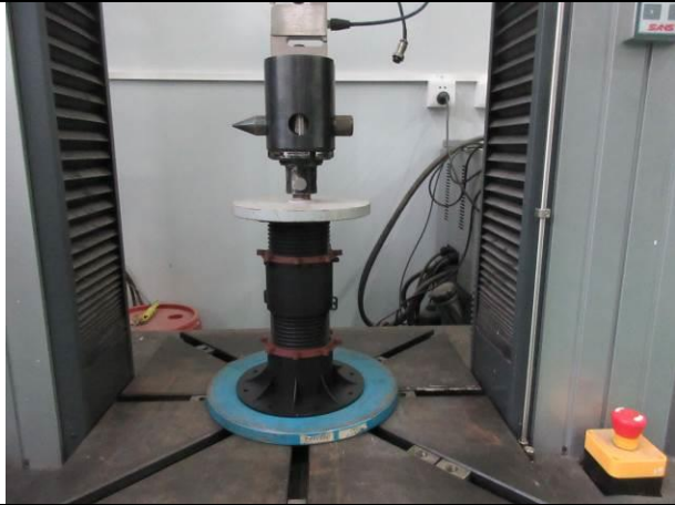
6. Over view of test setup for applying load on full section of upper surface of sample MT-DP-A1-A
