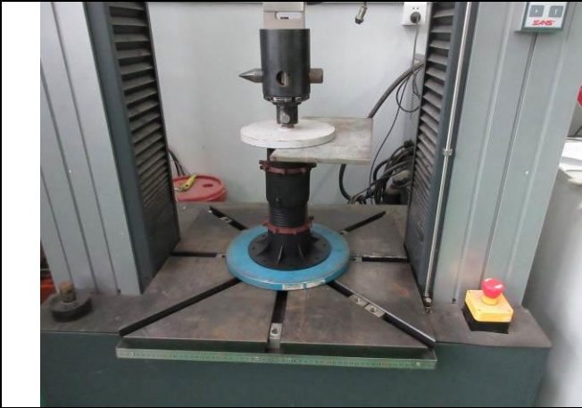
7. Over view of test setup for applying load on half section of upper surface of sample MT-DP-A1-A
