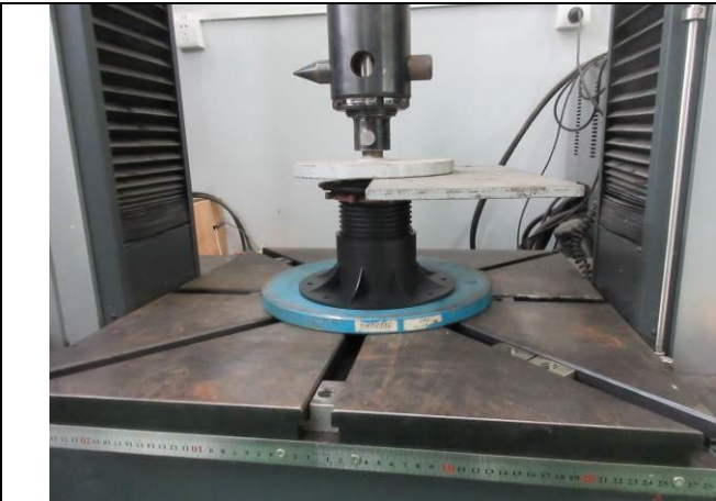
3. Over view of test setup for applying load on half section of upper surface of sample MT-DP-A0-A
