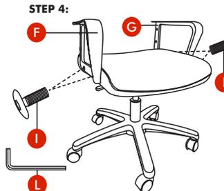
Note 1: Arm rests are labeled with an "L" (left) or "R" (right) to show which sides they should be placed on.
