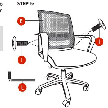
**Step 6:** Adjust the balance on each side of the chair, and fully tighten all the bolts to 100% at this step.
